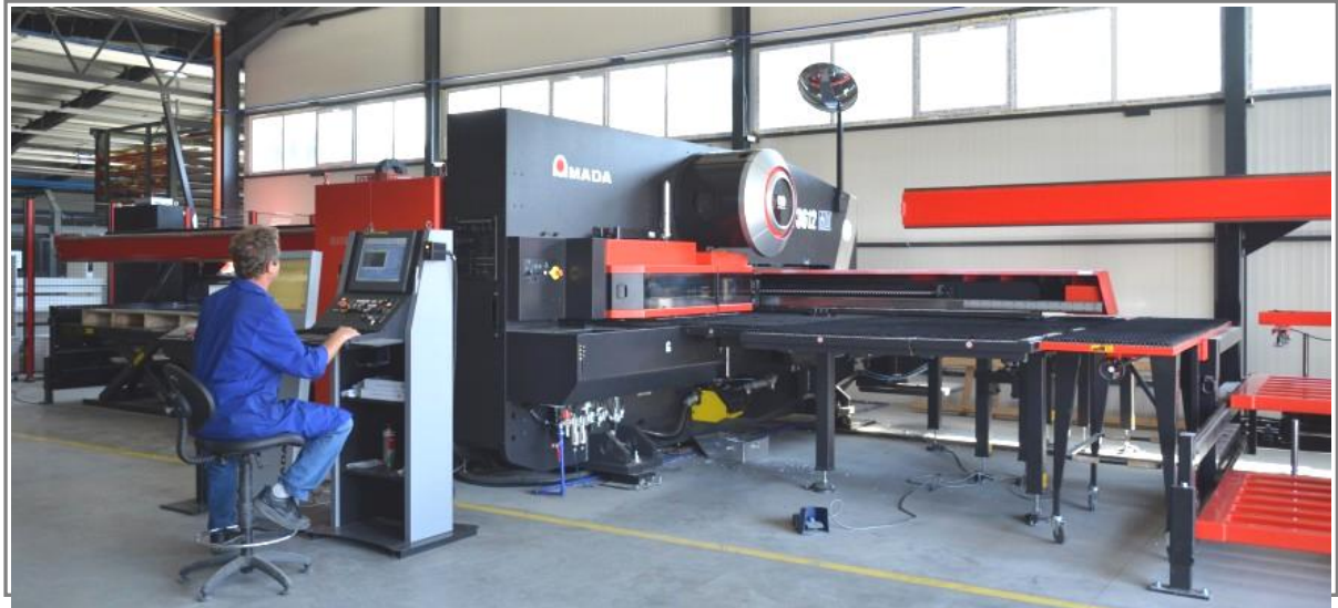
Revolver System: the revolver tool holder system “turret-shaped tool holder” allows up to 44 tools.
