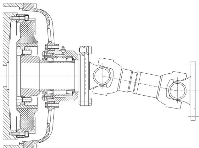
Every cardan shaft creates axial and radial reaction forces. The amount depends - among other reasons - on the transmitted torque and the operating angle. Under considerable operating angle these forces can become dangerous to the crankshaft of the diesel engines.
