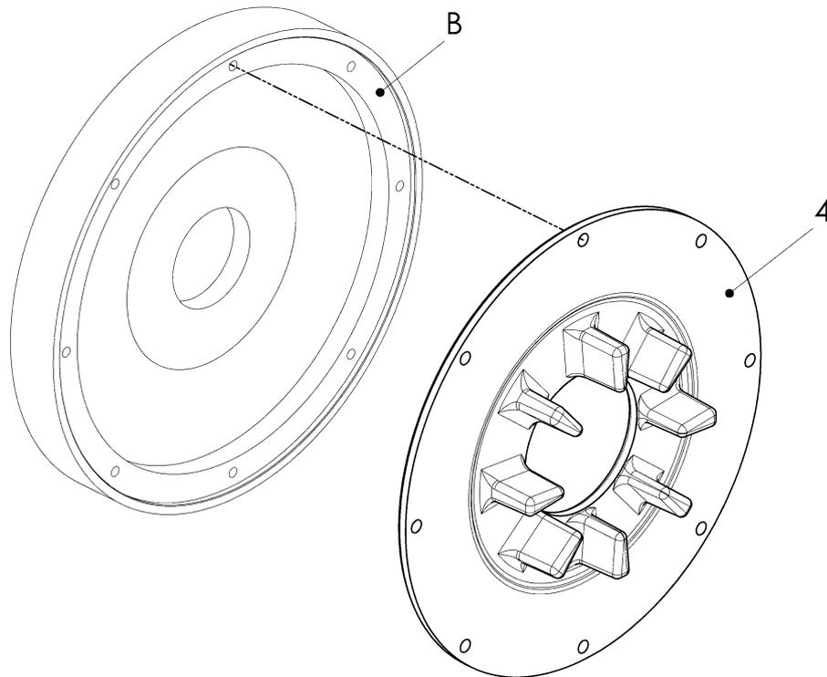
*Fig. 6-5 Mounting the inner part (4)*
