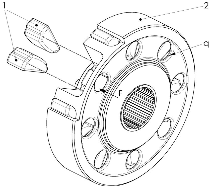
*Fig. 6-2 Preparing the outer part (2) with CENTA-conical clamping for mounting*
