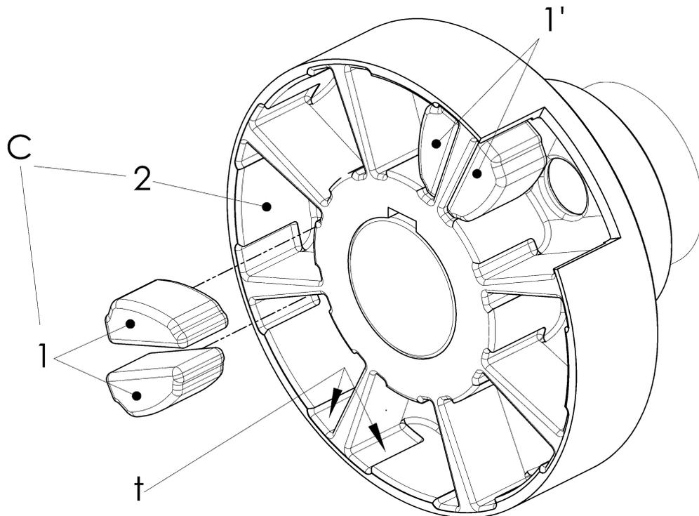
Fig. 6-4 Mounting the rubber elements
