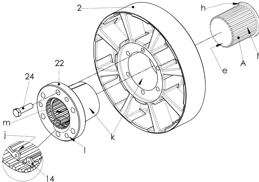
*Fig. 6-3 Mounting the outer part (2) with CENTA-conical clamping*
