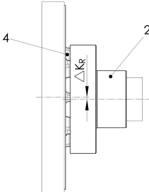
Fig. 5-2 Radial misalignment
