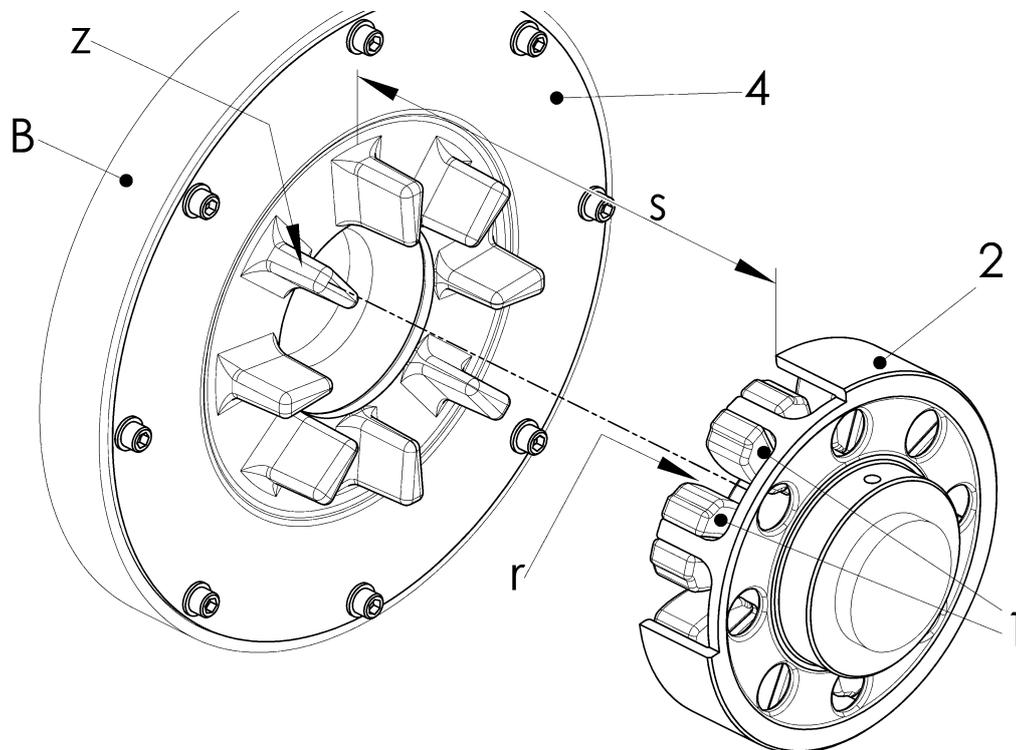
Fig. 6-6 Connecting the driving and driven units
