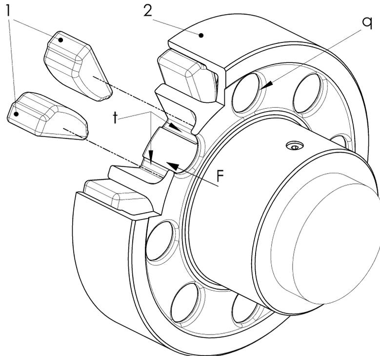
Fig. 9-1 Replacing the rubber elements (1)
