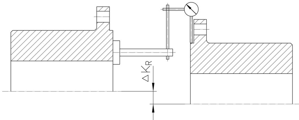
Fig. 5-2 Radial misalignment
