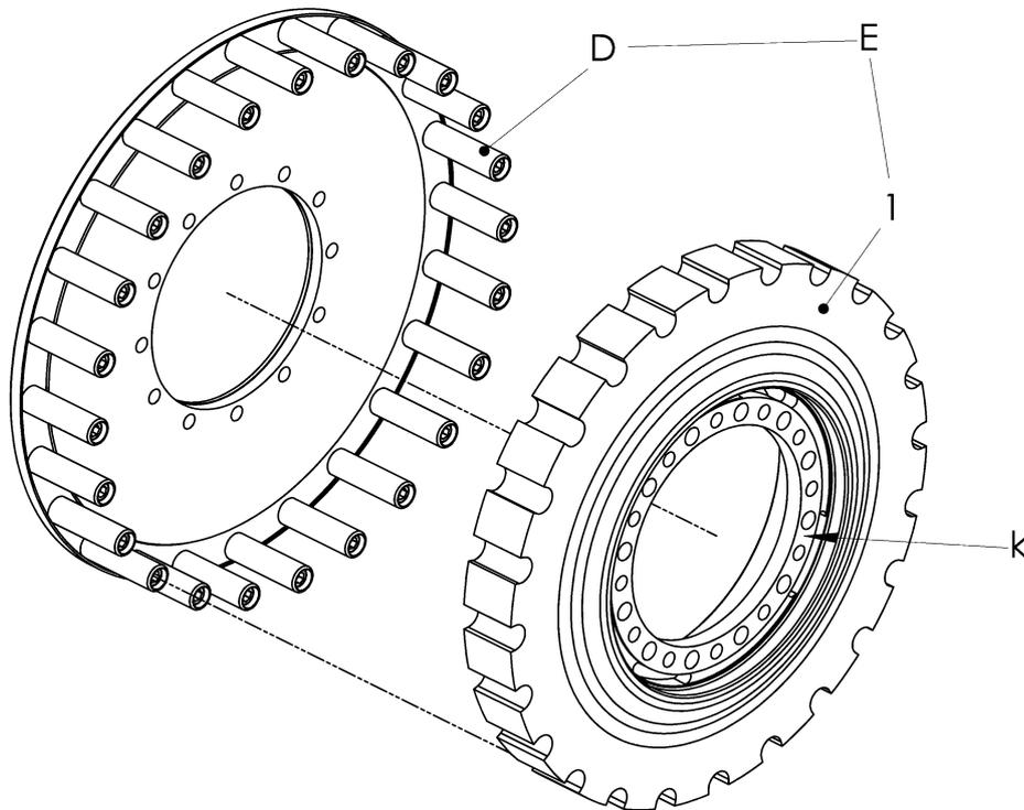
Fig. 6-5 Positioning the rubber element into the pre-mounted assembly (D)
