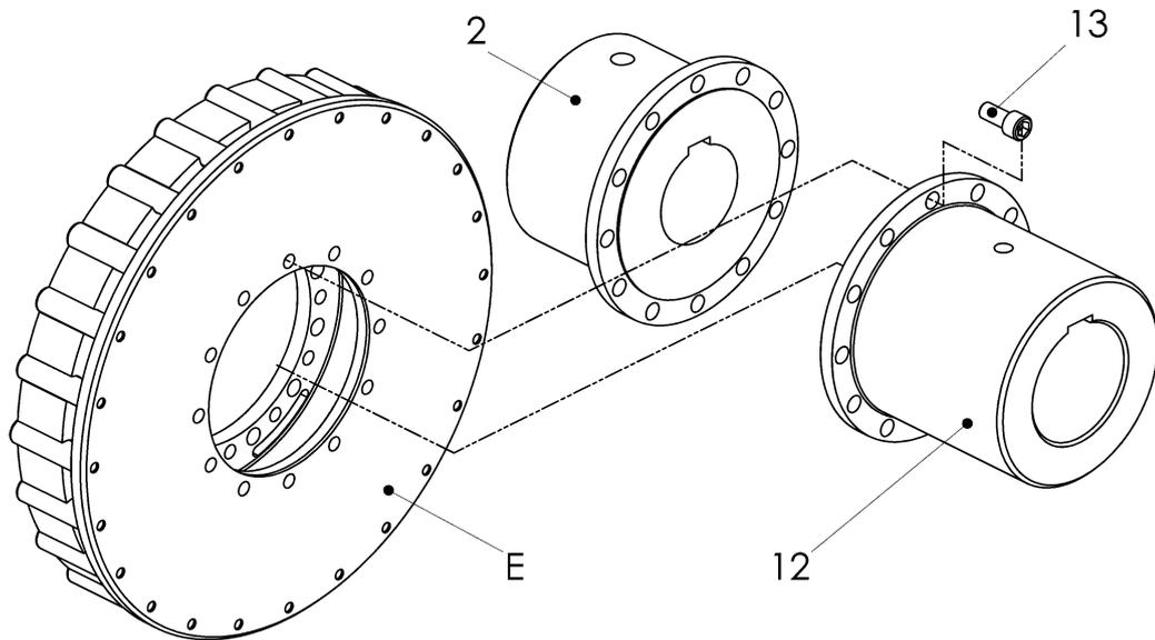
Fig. 6-6 Mounting the pre-mounted adapter with rubber element (E)
