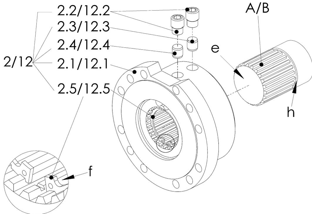
Fig. 6-4 Mounting the CENTALOC clamping hub
