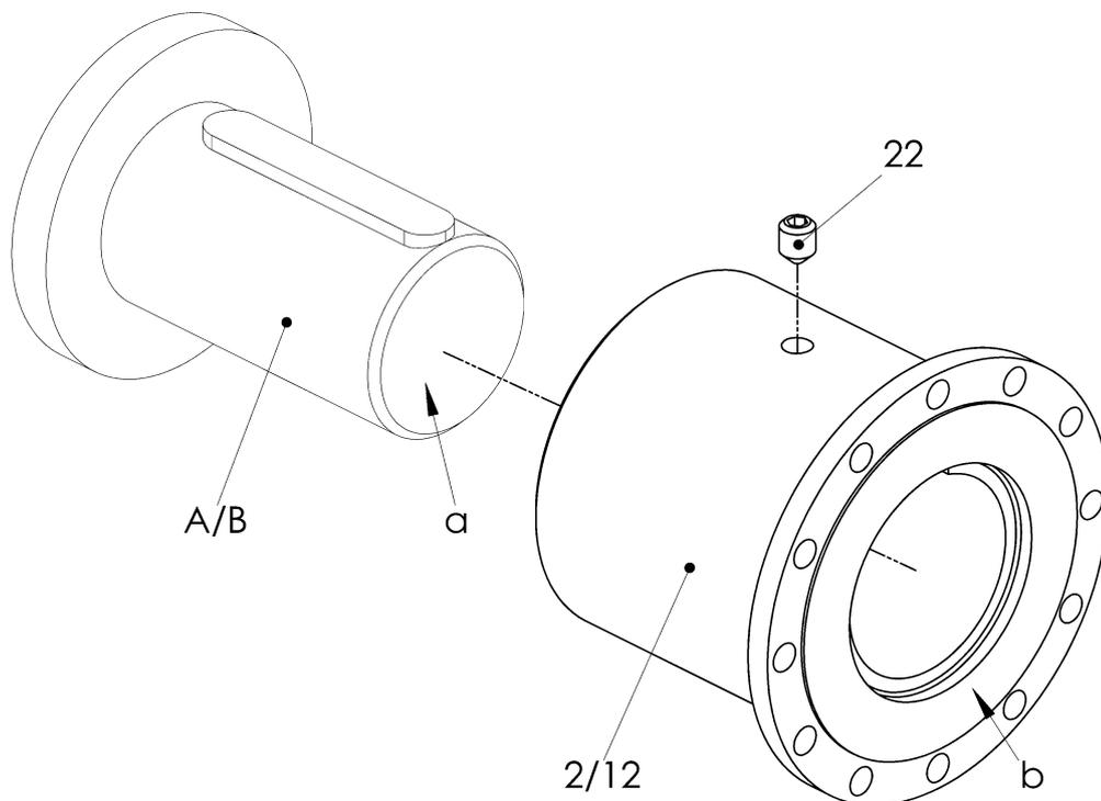
Fig. 6-1 Mounting the hub with cylindrical bore and keyway
