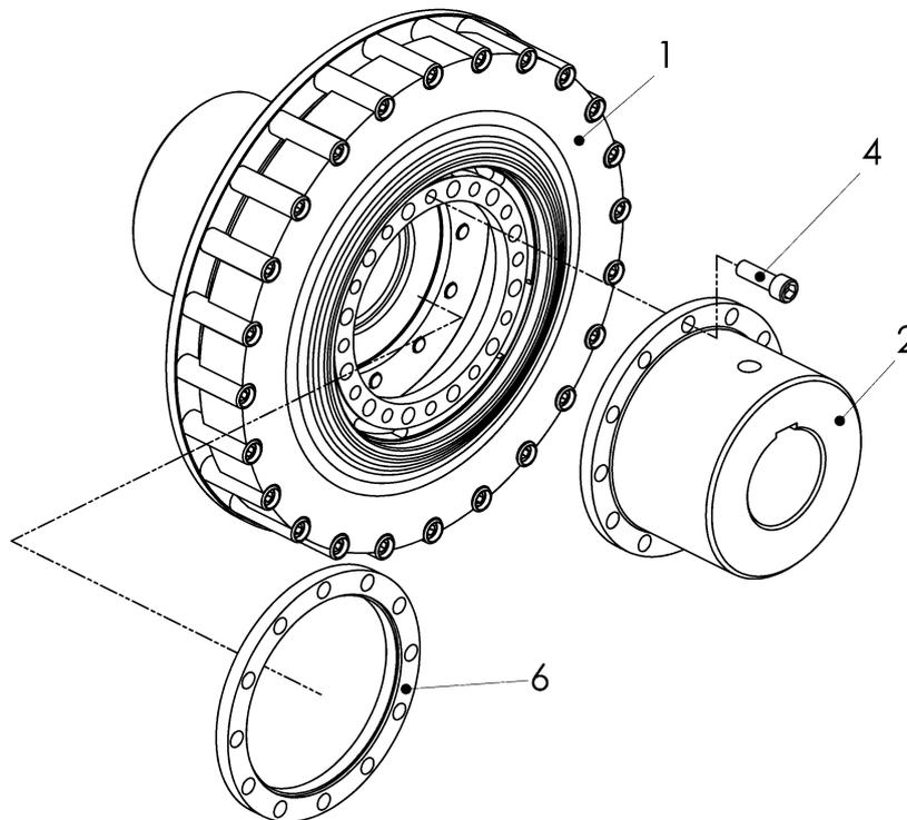
*Fig. 6-8 Mounting the rubber element (coupling sizes 5000 and 7000)*
