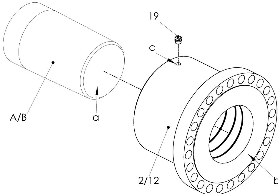
*Fig. 6-2 Mounting the hub with conical oil interference fit*
